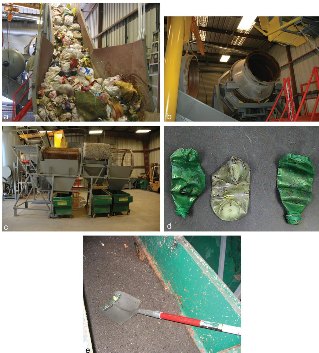
**Figure 1** Photographs of PET bottles reclaimed from MSW by vacuum-assisted steam autoclaving. [Color figure can be viewed in the online issue, which is available at [wileyonlinelibrary.com](http://wileyonlinelibrary.com).]
