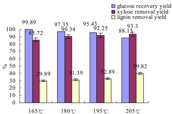
Fig. 6 – Effect of the temperature on the main components of almond shell after HWP (temperature from 165 °C to 205 °C).
