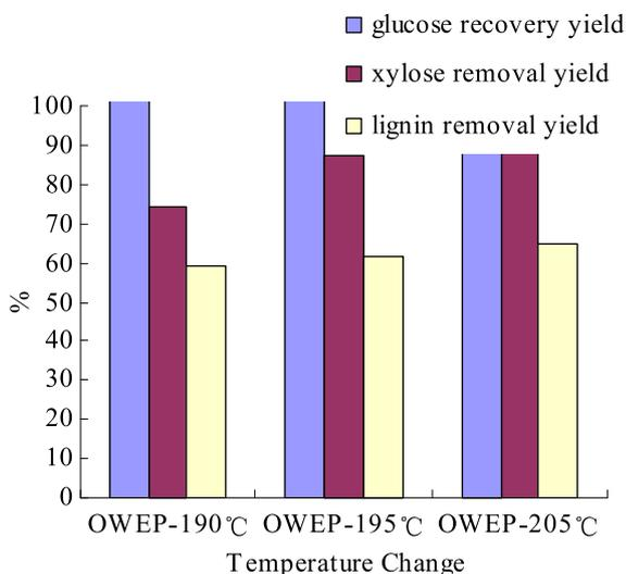
Fig. 7 – Effect of temperature on the compositions of almond shell in the second step OWEP (feedstock from the first-stage pretreatment HWP, ethanol in water mixtures of  $\langle \phi \rangle$  ethanol = 45% for 30 min).
