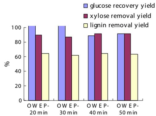
Fig. 8 – Effect of the time on the composition of almond shell in the second step of OWEP (195 °C, ethanol in water mixtures of  $\langle \phi \rangle$  ethanol = 45%).
