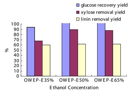
Fig. 9 – Effect of ethanol concentration on the composition of almond shell in the second step OWEP (195 °C, 20 min).
