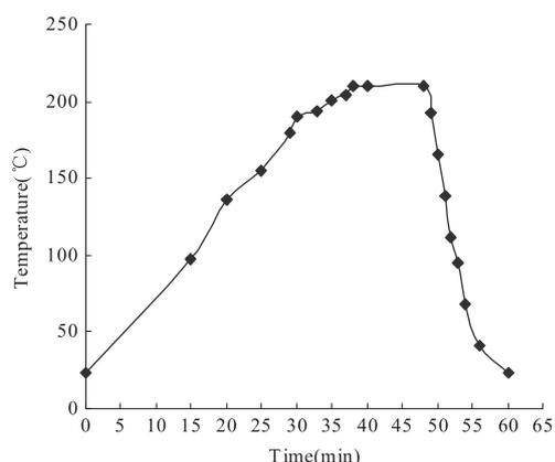
**Fig. 1 – Temperature change curve (The time of raising temperature was controlled in 30 min. The cooling time was controlled in 10 min. The time of thermal retardation was in according with the requirement of every experiment.).**
