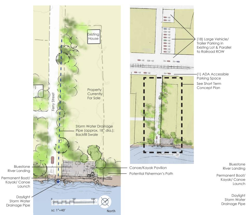
Bluestone **River** Landing 5 6 DAG Kayak/ Canoe Launch 50 Daylight ==== Storm Water Drainage Pipe sc: 1"=40'
